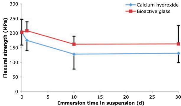
**Fig. 2.** Line graph depicting the changes in mean FS of standardized human root specimens ( $n = 20$  specimens per group) immersed in either a calcium hydroxide or a bioactive glass 45S5 suspension over time. Error bars indicate standard deviations.
