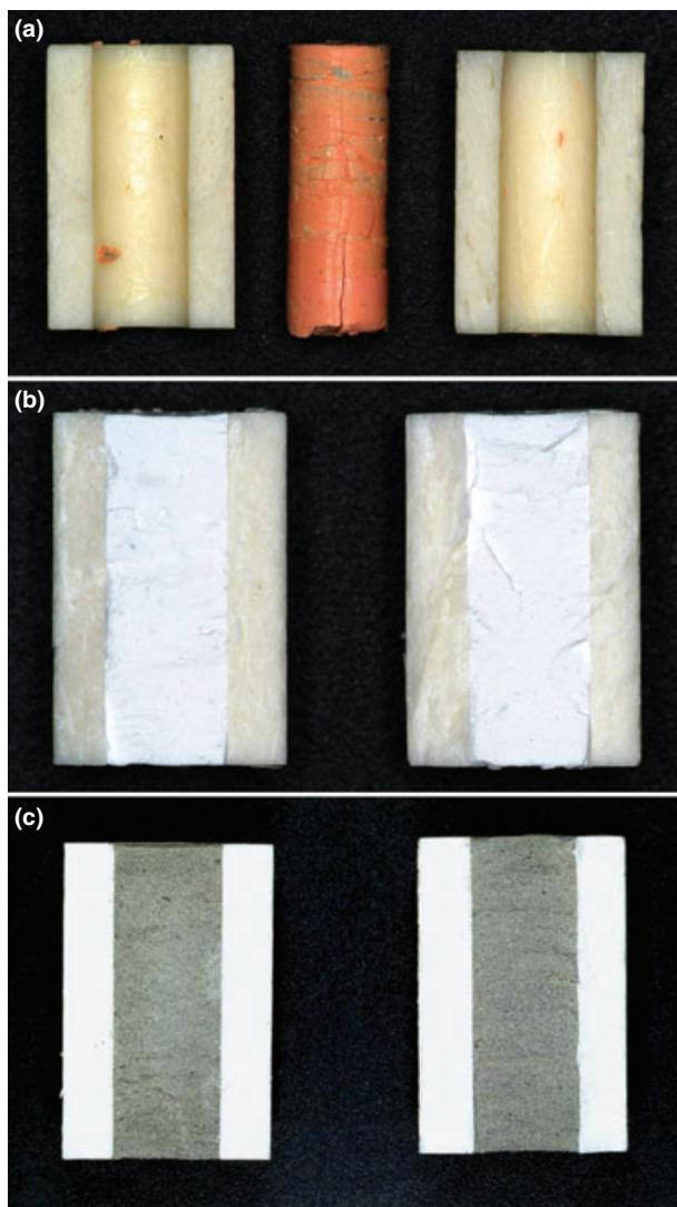
Fig. 2. Fractured samples of a thermoplasticized gutta percha (WGP) obturated bone cylinder (a), a calcium phosphate bone cement (CPBC) obturated bone cylinder (b) and a MTA obturated bone cylinder (c). Gutta percha (GP) detaches completely while CPBC and MTA adheres to the bone surface following pressure until ultimate force to fracture (UFF).
