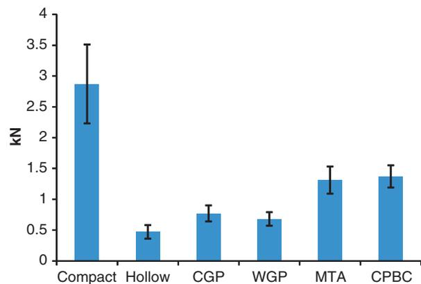
**Fig. 1.** The global mean and corresponding SD of the Ultimate Force to Fracture (UFF) for the different treatments (compact, hollow, lateral gutta percha condensation CGP, thermoplasti-cized gutta percha WGP, MTA and calcium phosphate bone cement CPBC).
