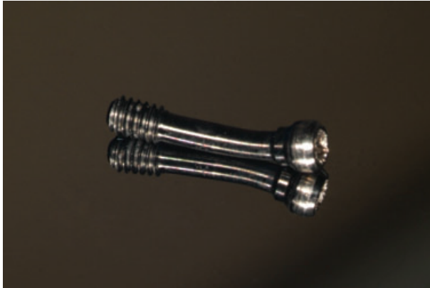
Fig. 4. Bent fixation screw.
