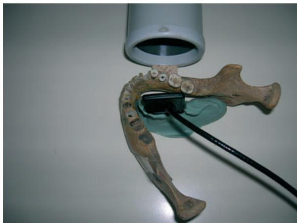
Fig. 1. CCD sensor was placed in putty material for fixed placement of the sensor in a standard position for imaging of each specimen.
