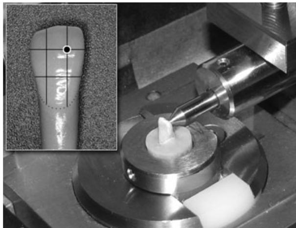
Fig. 1. Specimen mounted on the test jig to perform fracturing load. Inset: Point for application of perpendicular fracture loading.
