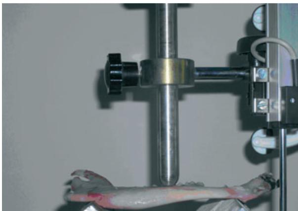
Fig. 1. Three-point bending test.
