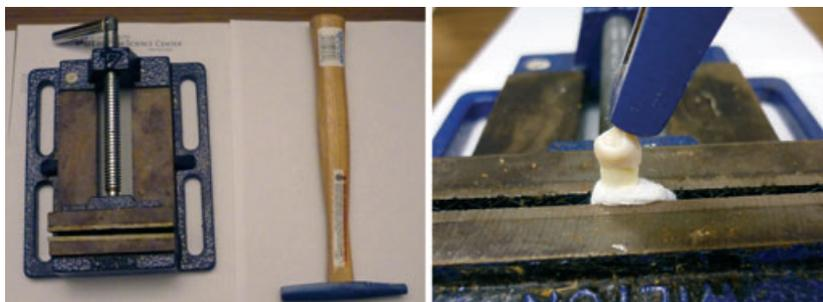
Fig. 1. Device used in creating the artificial root fractures.
