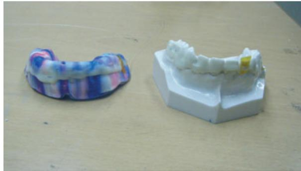
Fig. 10. Fiber Bragg Grating sensor surface mounted on the mouthguard and typhodont using EA-2A Epoxy resin Adhesive.
