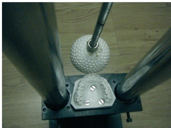
Fig. 2. Ball apparatus hitting the most prominent tooth on the typhodont model.
