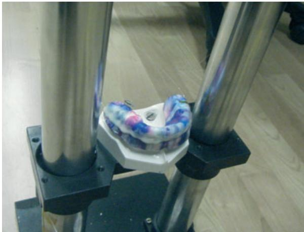
Fig. 12. The typhodont along with mouthguard with Fiber Bragg Grating sensor mounted secured to the base of the pendulum apparatus using screws.
