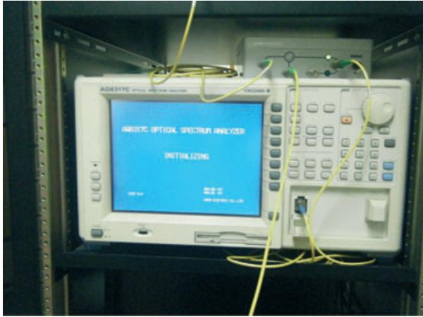
Fig. 11. Interrogator: Optical spectrum analyzer (OSA) used for measuring wavelength shift in fibre bragg grating sensor.
