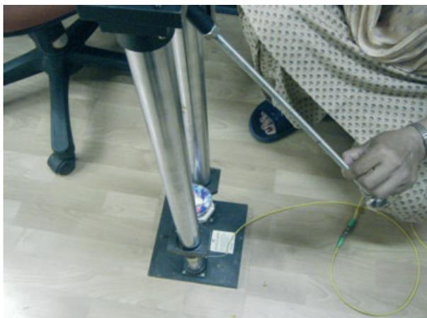
Fig. 14. Impact Release from height H2 = 48 cm from ground level.
