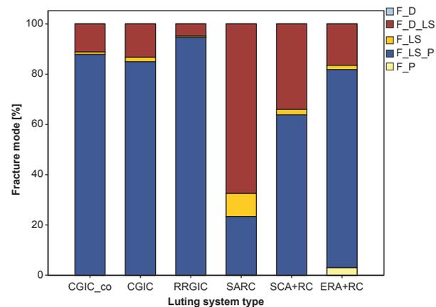
Fig. 4. Failure mode analysis [%] of conventionally and adhesively luted posts to bovine root canal dentin, depending on the luting system type. CGIC\_co, conventional glass-ionomer cement; control with titanium post; CGIC, conventional glass-ionomer cement; RRGIC, resin-reinforced glass-ionomer cement; SARC, self-adhesive resin cement; SCA + RC, self-conditioning adhesive + resin cement; ERA + RC, etch and rinse adhesive + resin cement.
