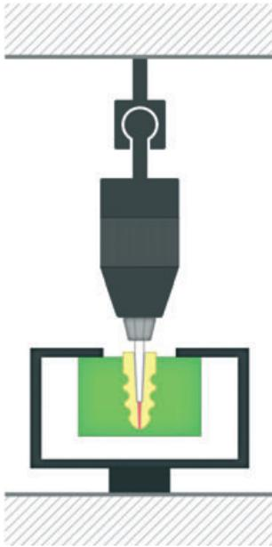
Fig. 1. Schematical illustration of the pull-out test design.
