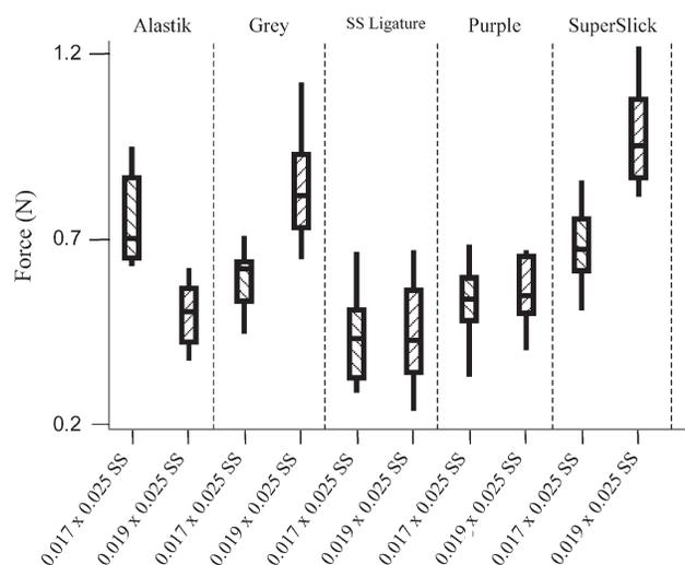
**Figure 3** Boxplots for mean frictional force by method of ligation for 0.017 × 0.025 and 0.019 × 0.025 inch stainless steel wires.
