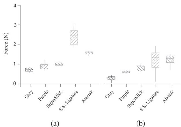
**Figure 2** Boxplots for median archwire seating force by method of ligation for (a) 0.017 × 0.025 and (b) 0.019 × 0.025 inch stainless steel wire.
