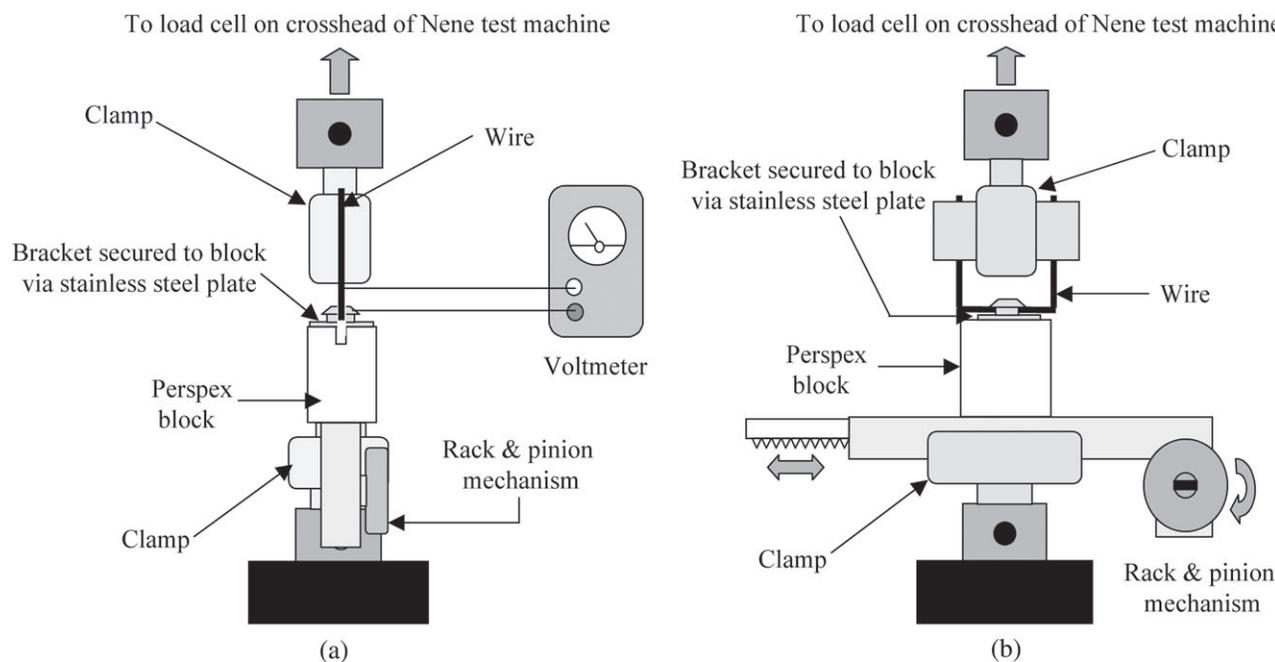
**Figure 1** Diagrammatic representation of the experimental set-up: (a) side view and (b) front view (syringe not shown).
