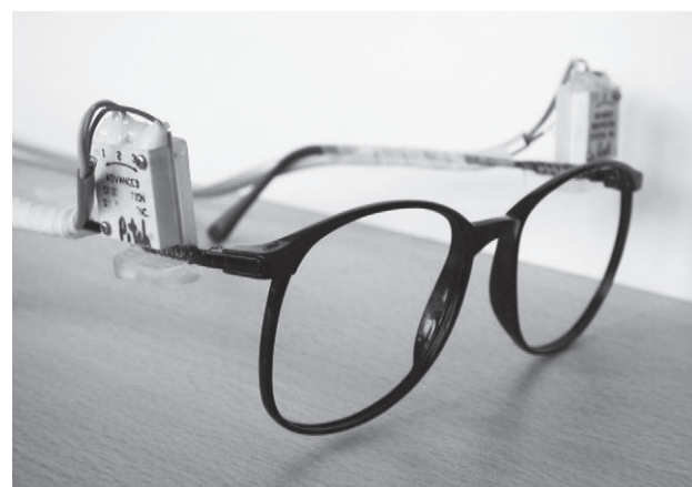
Figure 2 Cranial portion of the device. Note the placement of inclinometers on opposite sides.
