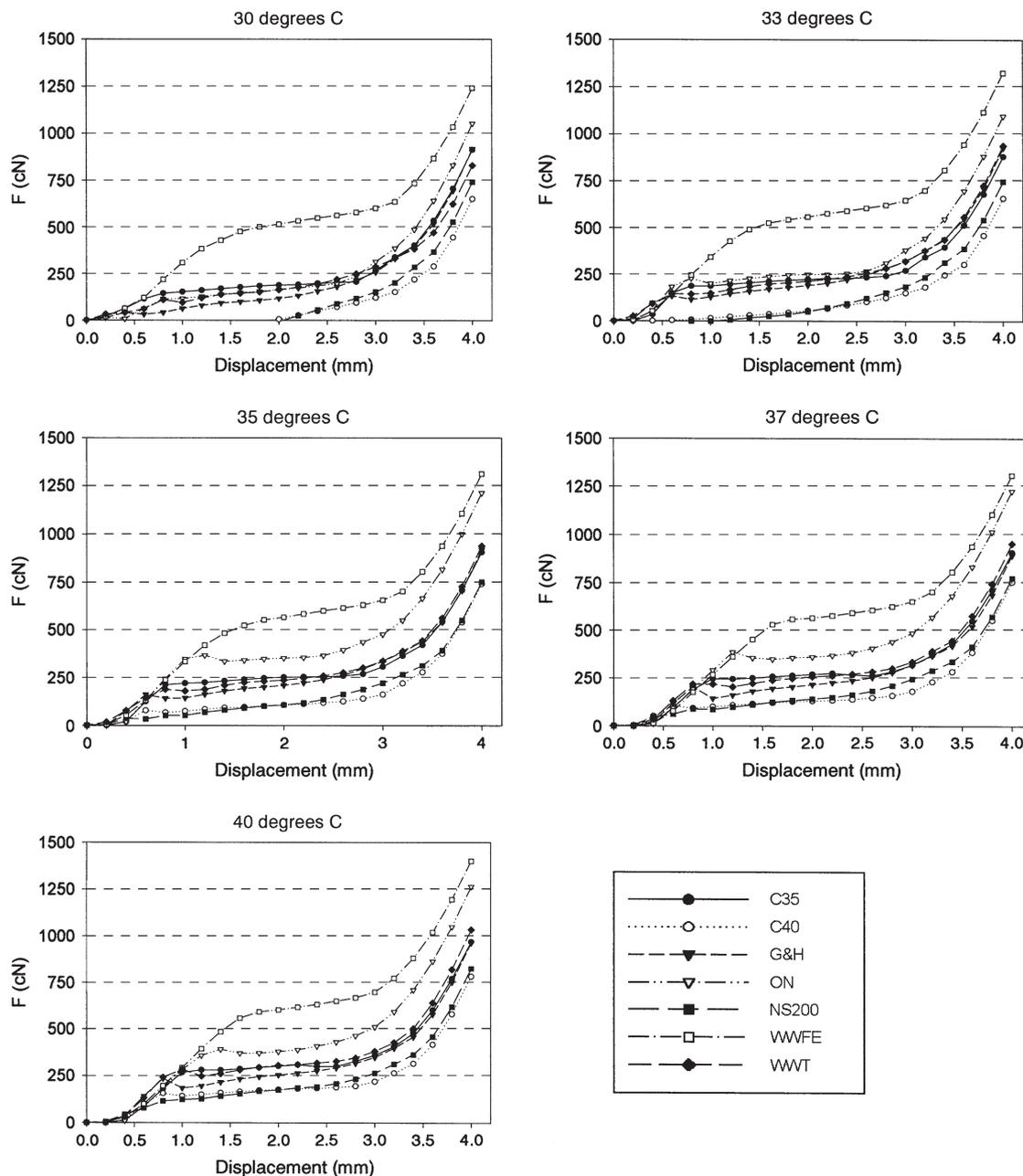
**Figure 4** Unloading curves of the tested archwires at the five different temperatures. (See Table 2 for definitions of abbreviations.)
