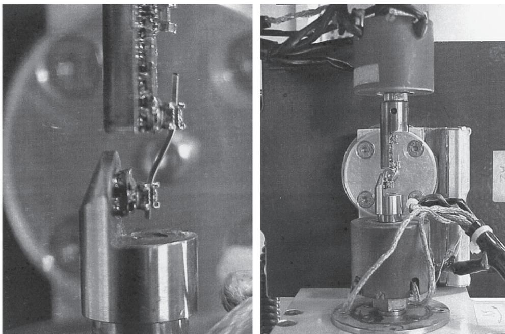
**Figure 1** Force System Identification apparatus with two self-ligating Damon brackets testing the wire in first order activation.
