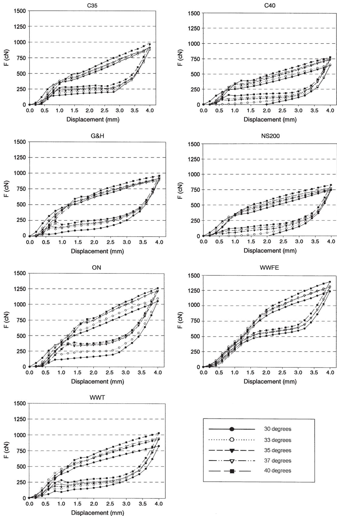
Figure 3 Temperature-dependency of the seven different brands of archwires. (See Table 2 for definitions of abbreviations.)
