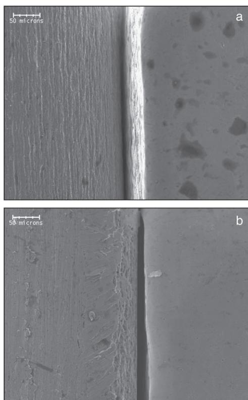
**Figure 2** Scanning electron microscopy photomicrographs ( $\times 200$ ) of coupling of (a) NiTi wire and FeCrNi bracket, and (b) CuNiTi wire and FeCrNi bracket in Fusayama-Meyer saliva.
