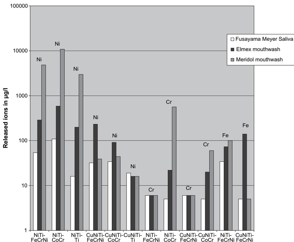
**Figure 1** Metal ions (in µg/l) released by wire-bracket combinations in the different solutions.
