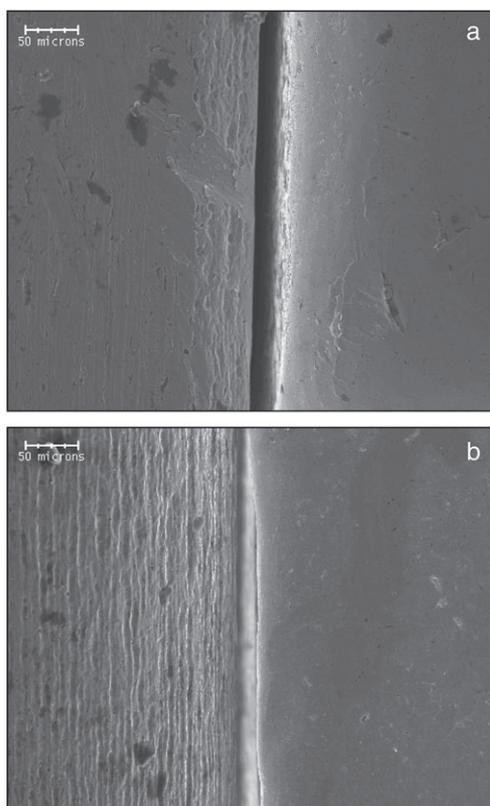
**Figure 3** Scanning electron microscopy photomicrographs ( $\times 200$ ) of coupling of (a) CuNiTi wire and FeCrNi bracket, and (b) NiTi wire and FeCrNi bracket in Elmex® mouthwash.
