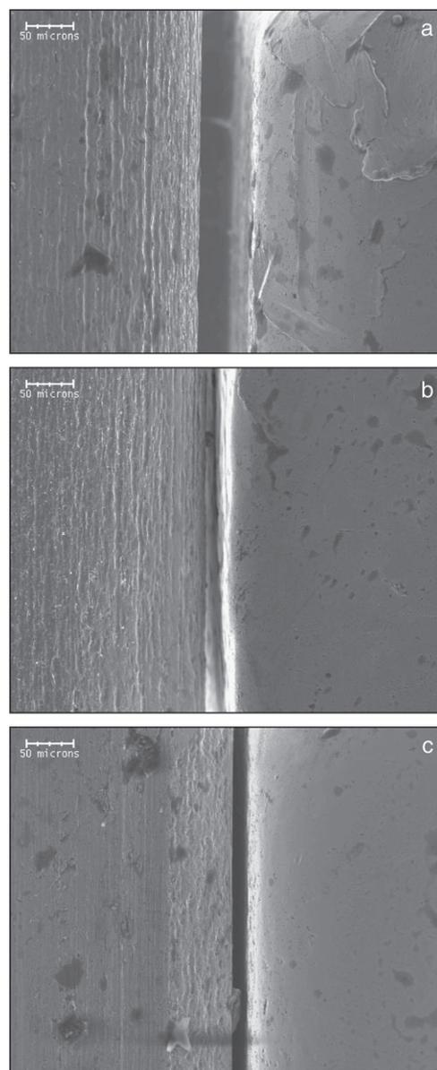
**Figure 4** Scanning electron microscopy photomicrographs ( $\times 200$ ) of coupling of (a) NiTi wire and CoCr bracket, (b) NiTi wire and FeCrNi bracket, and (c) CuNiTi wire and CoCr bracket in Meridol® mouthwash.
