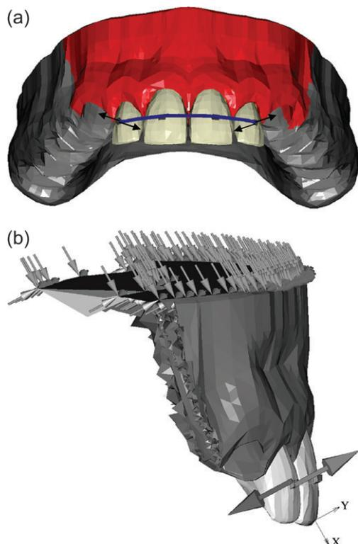
**Figure 4** (a) Finite-element (FE) model of the maxilla with the four anterior teeth. Arrows indicate the force couples. Only the anterior part of the model was used for the calculations. (b) Orthogonal view of the anterior part of the FE model. The force couples are indicated by the arrows at the lateral incisor bracket. Boundary conditions are indicated by the arrows on top of the model. All three translational degrees of freedom of the nodes on the outer surface of the bone are fixed.
