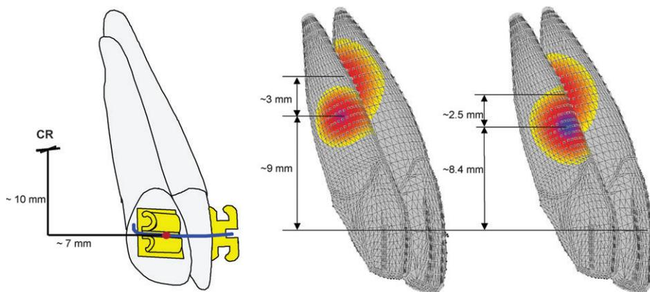
**Figure 7** With increasing rigidity of the stabilizing archwire (right side: wire cross-section  $1.38 \times 1.92 \text{ mm}^2$ ), the individual centres of resistance (CRs) move closer to each other.
