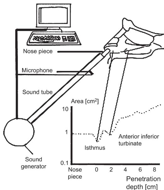
Figure 1 Diagram of the acoustic rhinometry device.
