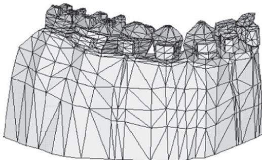
**Figure 2** Oblique view of the three-dimensional finite element model of the lower right dentition. The model consists of the teeth, periodontal membrane, alveolar bone, and brackets.
