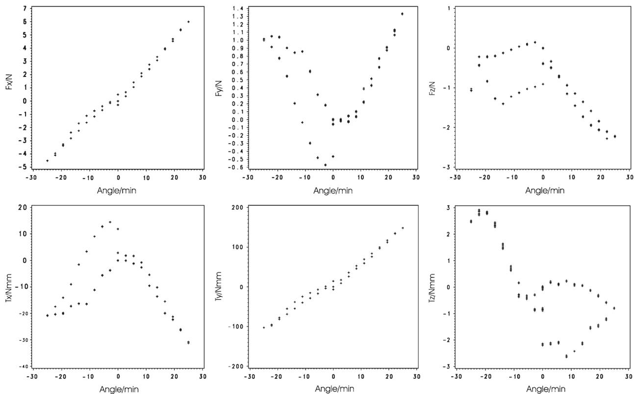
**Figure 2** Typical forces ( $F_x$ ,  $F_y$ , and  $F_z$ , upper row) and moments ( $T_x$ ,  $T_y$ , and  $T_z$ , lower row) in the present study as a function of the magnitude of displacement of the tooth measured for one material (Biolon®).
