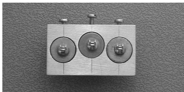
Figure 1 Set-up including three passive self-ligating brackets. The tested brackets were individually bonded to a brass mount using a preformed 0.021 × 0.025 inch stainless steel wire jig in order to exclude adverse tipping or torsion moments.
