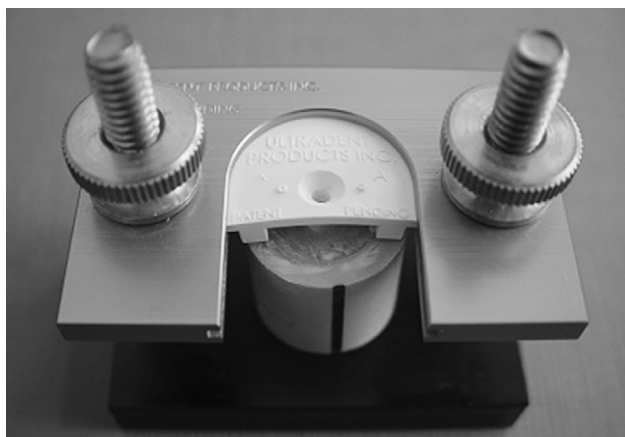
Figure 1 Device used for placing standard composite blocks on enamel surface.
