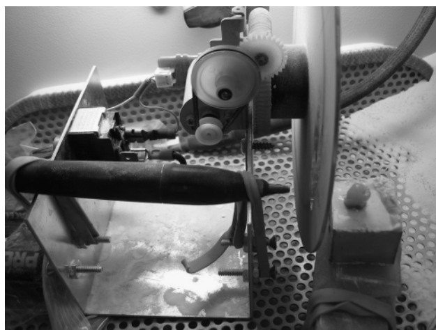
Figure 1 Mounted tooth undergoing air abrasion treatment through the aperture of rotating wheel.
