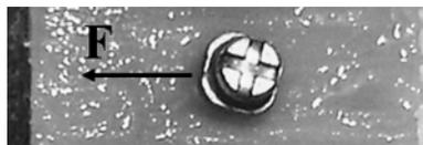
**Figure 2** Mini-implant inserted in a bovine bone segment. The force axis was parallel to the bone surface and perpendicular to the long axis of the animal rib.
