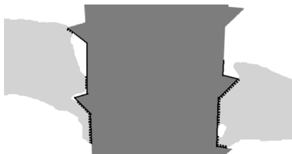
Figure 3 Method used to measure the bone-implant contact ratio. The bone-to-implant contact ratio equals the length of bone contact with cortical bone (dashed line) divided by the length of the mini-implant surface at the cortical bone \times 100 .
