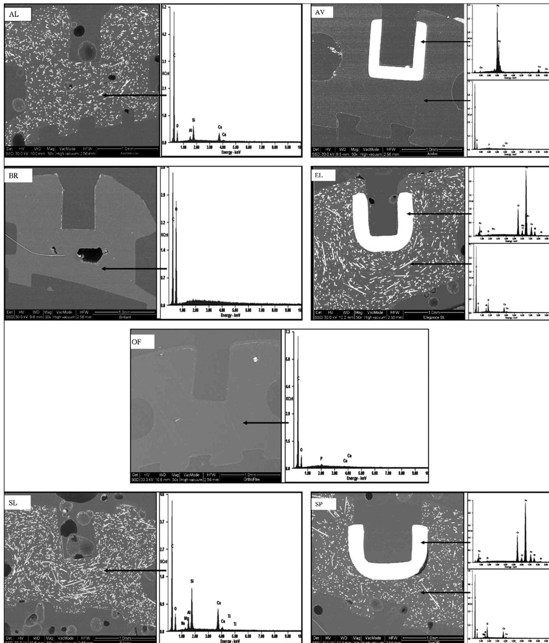
**Figure 3** Compositional backscattered electron images (SSD,  $\times 50$  magnification) of cross-sectioned bracket specimens and energy-dispersive X-ray spectra of bulk materials and metallic slots.
