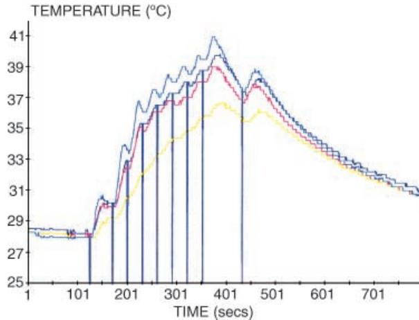
**Figure 3** A typical tracing of temperature recorded versus time by thermocouples placed at the mid-root level. (Each of the thermocouples is represented by a single colour line, the blue vertical lines mark the beginning of each ultrasonic activation).
