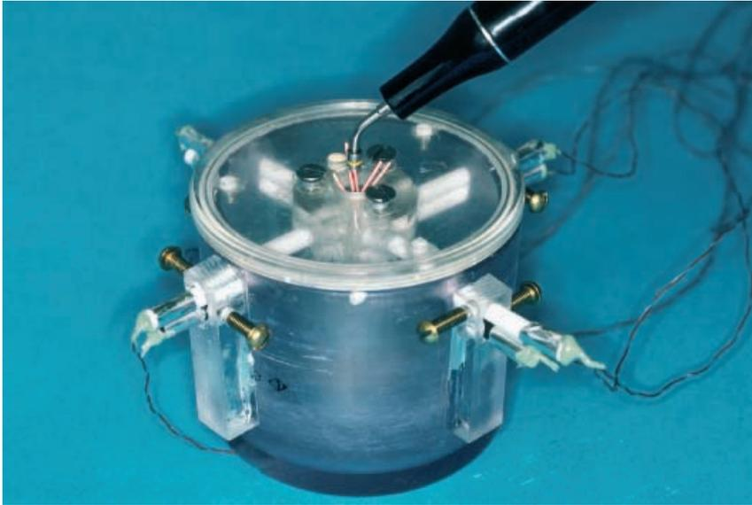
**Figure 2** The tooth/ acrylic cylinder assembly placed inside the plastic draft and temperature insulator.
