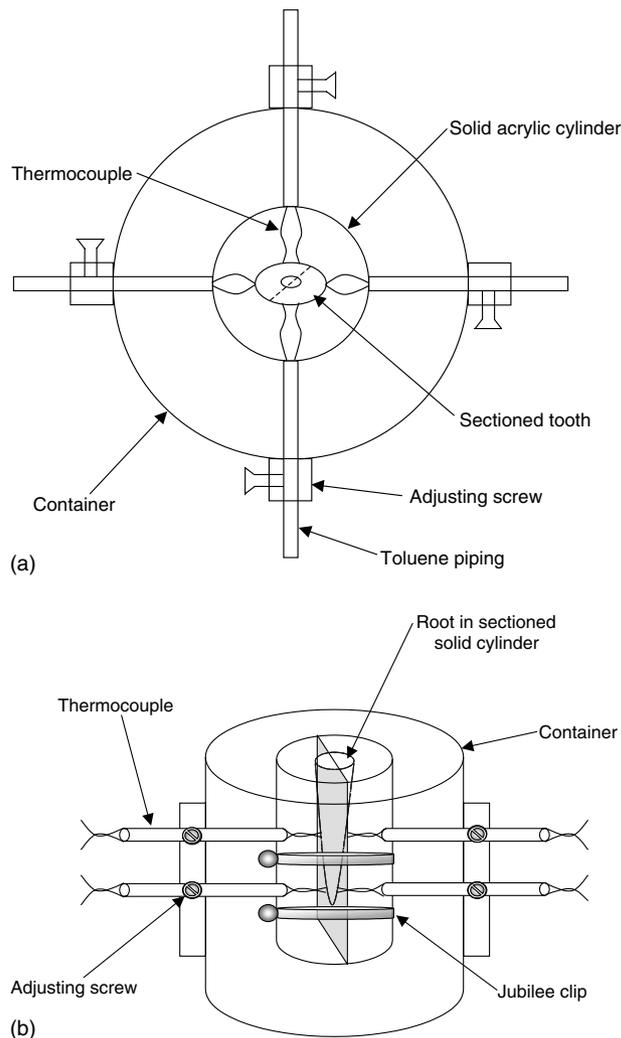
**Figure 1** Schematic diagram of the temperature measurement apparatus viewed in longitudinal and transverse sections.
