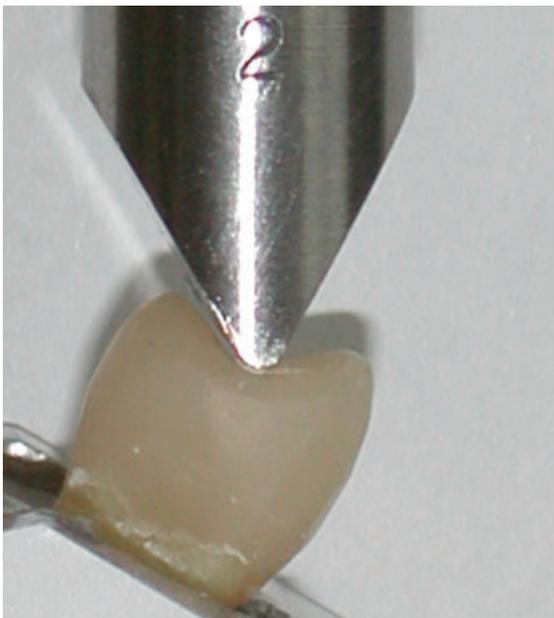
**Figure 1** Position of a specimen with a direct resin composite complete crown in the test set-up for static loading.
