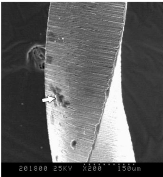
**Figure 3** Photomicrograph of a discarded S1 instrument showing the presence of surface debris (arrow) and substantial 'roll-over' at the cutting edge.
