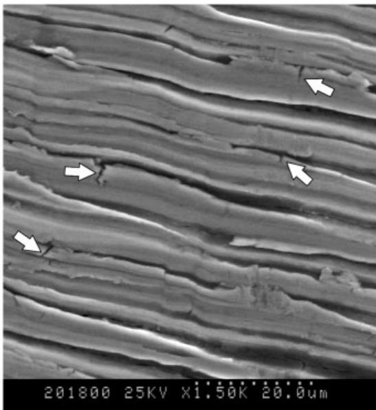
**Figure 5** Photomicrograph of an intact, discarded S1 instrument at the 3.1–4.1 mm region from the tip showing the presence of microcracks (arrows) running perpendicular to the machine grooves on the instrument surface. Tip of the instrument was towards the upper edge of the picture.
