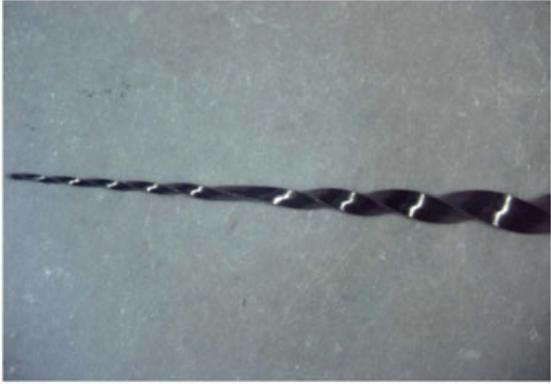
**Figure 2** Discarded file showing unwinding defects without fracture.
