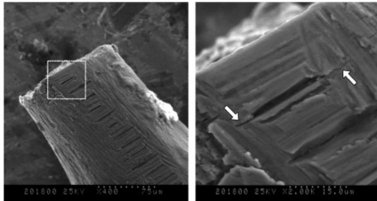
**Figure 8** Photomicrograph of an unwound but intact S1 instrument showing considerable defects at the unwound region, including pitting (a), microcracks (b), and severely distorted machine grooves (c).
