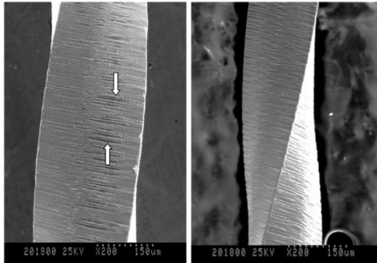
**Figure 7** Photomicrograph of a fractured S1 instrument showing the presence of surface cracks close to the fracture site.
