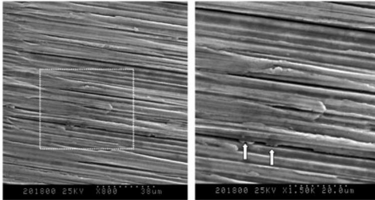
**Figure 4** Photomicrograph of an intact S1 instrument showing numerous machine grooves running near-parallel to one another (across the entire field) on its surface, and the presence of debris particles (arrows) within a crack-like structure at the 3.1–4.1 mm region from the instrument tip.
