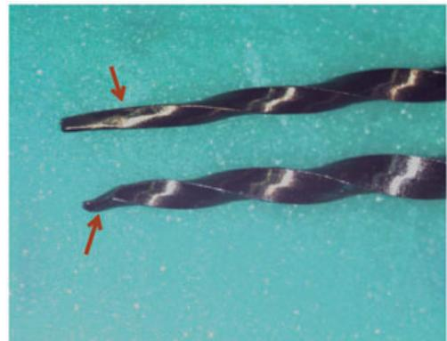
**Figure 1** Photograph of the two discarded, fractured S1 files with associated unwinding defects (arrows).
