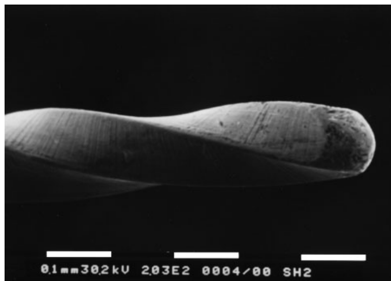
Figure 12 SEM picture of Shaping™ file tip (courtesy of Dr A. Butti and Dr N.M. Grande, Catholic University of Sacred Heart, Rome).
