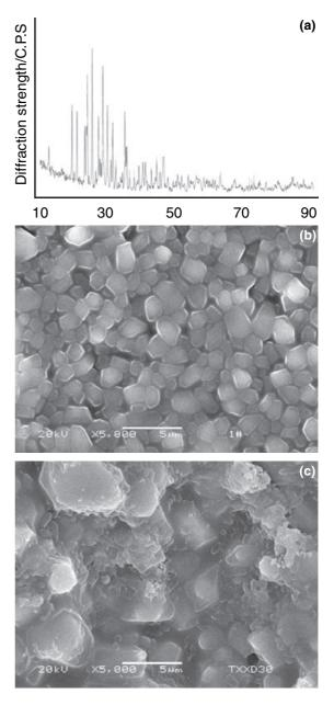
**Figure 1** Characterization of calcium polyphosphate (CPP). (a) X-ray diffractometry (XRD) analysis of CPP powder. The surface of original CPP (b) and that of CPP after 20 days degradation (c) was examined by SEM. Magnification: 5000×.
