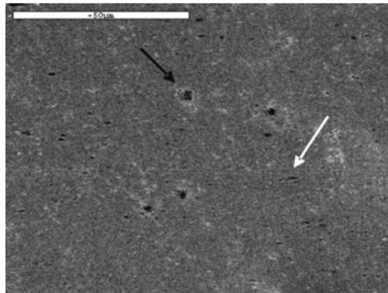
**Figure 4** Surface ( $\times 1000$ ) of longitudinal section of a Mani sample in the 'as-received' condition, with minimal roughness (level 1). Holes (black arrow) and inclusions (white arrow) randomly distributed within nickel–titanium matrix.
