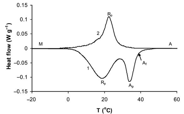
**Figure 7** Differential scanning calorimetry thermogram for the ‘as-received’ sample. 1, heating; 2, cooling.
