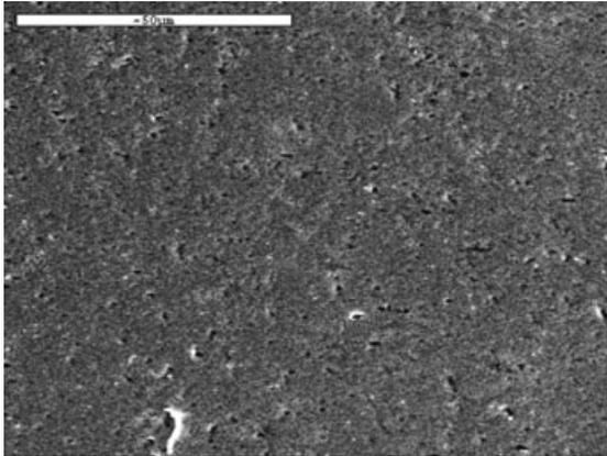
**Figure 5** Surface ( $\times 1000$ ) of longitudinal section of a Mani sample that was subjected to 11 sterilizations. Increased roughness of the surface (level 3) was the prevalent finding.
