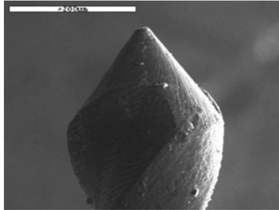
**Figure 3** Mani instrument after 11 sterilization cycles. Increased surface roughness (level 3) was evident.
