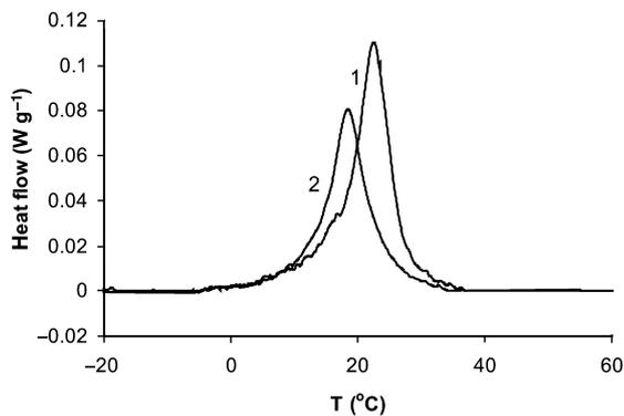
**Figure 9** Differential scanning calorimetry thermogram during cooling. 1, 'as-received' sample; 2, sample after 11 sterilization cycles.
