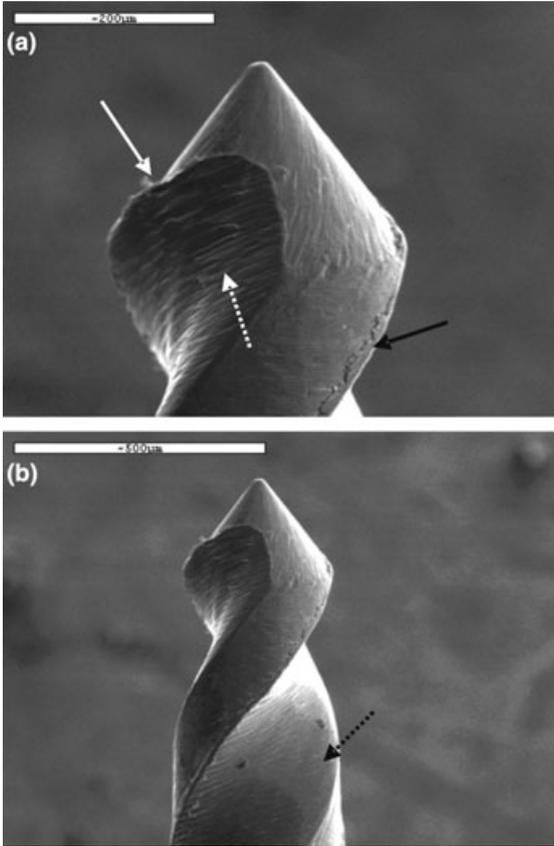
**Figure 1** Mani instrument in the 'as-received' condition, with rounded, noncutting tip. (a) Magnification  $\times 200$ , (b) magnification  $\times 75$ . Presence of debris (white arrow), metal strips (white distinct arrow), machining defects along the cutting edges (black arrow) and pits (black distinct arrow). The surface roughness was considered minimal (level 1).
