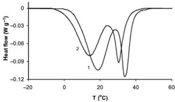
**Figure 8** Differential scanning calorimetry thermogram during heating. 1, 'as-received' sample; 2, sample after 11 sterilization cycles.
