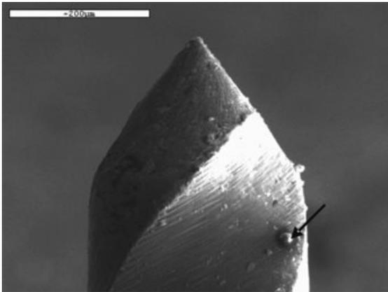
**Figure 2** Mani instrument in the 'as-received' condition, with sharp cutting tip. Debris is detected near the cutting edge of the file (black arrow). Moderate roughness of the surface (level 2) was observed.
