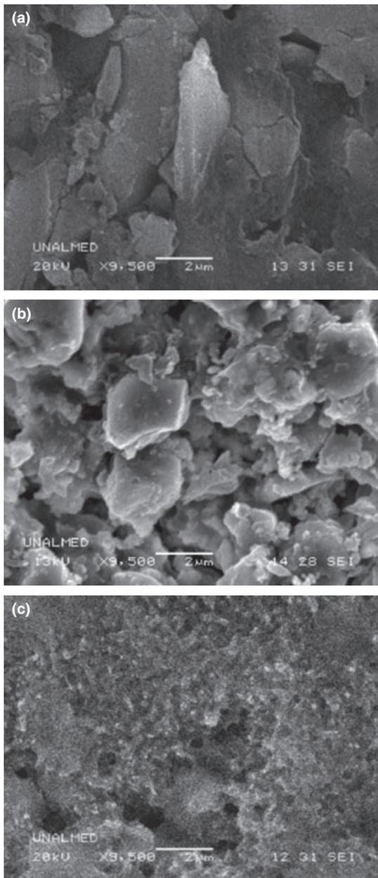
**Figure 4** Scanning electron micrographs of representative polished longitudinal sections of root-end fillings. (a) Surface of IRM showing closely packed and splinter-shaped interconnected crystals with some spaces on the split surface. (b) Structure of sEBA showing a rough surface composed of fine and coarse sphere-like merged microparticles. (c) Capillary structure of MTA; a highly fused surface texture is evident. Original magnification  $\times 9500$ .
