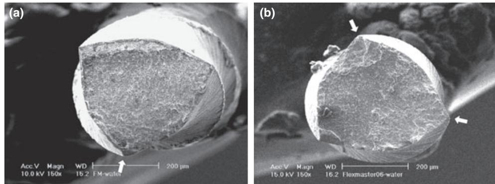
**Figure 6** (a, b) Photomicrographs of the fracture cross-section of FlexMaster instruments; crack origins are indicated (arrow).
