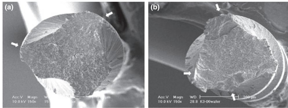
**Figure 4** (a, b) Photomicrographs of the fracture cross-section of K3 instruments; crack origins are indicated (arrow).
