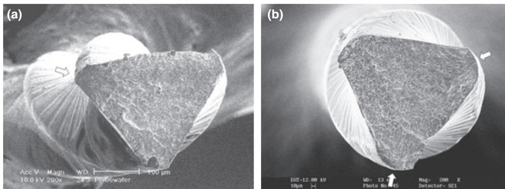
**Figure 3** (a, b) Photomicrographs of the fracture cross-section of ProFile instruments; crack origins are indicated (arrow).
