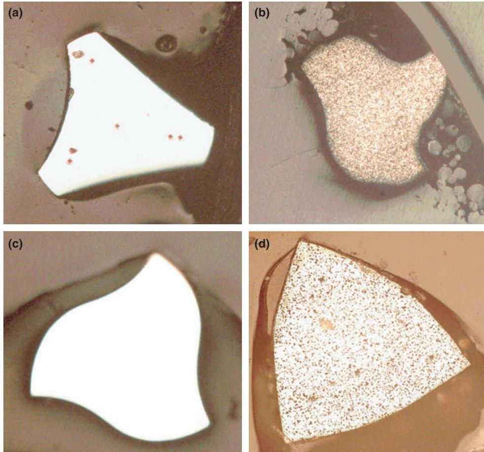
**Figure 1** Cross-sectional shape (at about 5 mm from the tip and polished) of four brands of instrument: (a) ProFile (Dentsply Maillefer, Ballaigues, Switzerland); (b) K3 (SybronEndo, Orange, CA, USA) (Note: strip on the right of field is a positioning holder); (c) HERO Shaper (Micro-Mega, Besançon, France); (d) FlexMaster (VDW, Munich, Germany).
