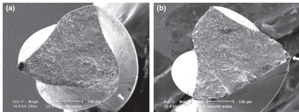
**Figure 5** (a, b) Photomicrographs of the fracture cross-section of HERO Shaper instruments; crack origins are indicated (arrow).
