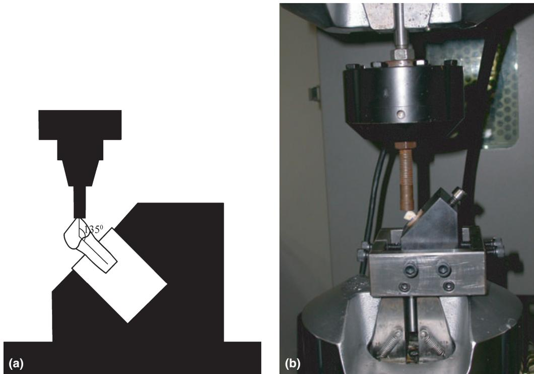
**Figure 2** (a) Cylindrical device used for fixation and positioning of specimens subjected to fracture strength testing. Device positioned for load application at 135°. (b) Load being applied on the buccal surface.
