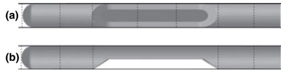
**Figure 1** Verification of the cylindrical shape of the specimens during the preliminary study. (a) Needle outlet orientated towards the magnifying lens. (b) Needle outlet at right angle to the lens. Specimen external diameter was determined as the length of the dashed lines in 15 equally spaced points. Only a part of the specimen was included in the figure for illustration purposes.
