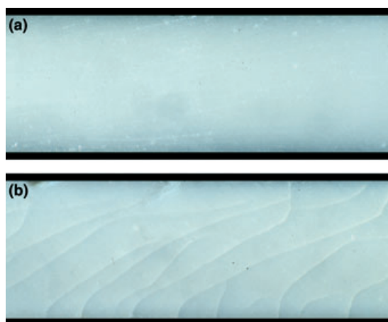
Figure 4 Macrophotograph depicting a dentin bar that was immersed in water (a) and a counterpart that was immersed in 5% NaOCl (b) for 2 h. Not after 1 h (cf. Results section), but after 2 h immersion in 5% NaOCl (b), spontaneous cracking of the dentine surface could be observed macroscopically ( n = 3 per group).
