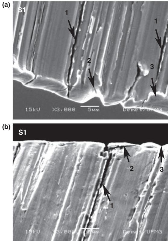
**Figure 1** Typical crack patterns in S1 instruments used for cleaning and shaping (a) five molars (group A) and (b) eight molars (group B). Arrows number (1) microcracks; (2) wear mark; (3) blunted edge.
