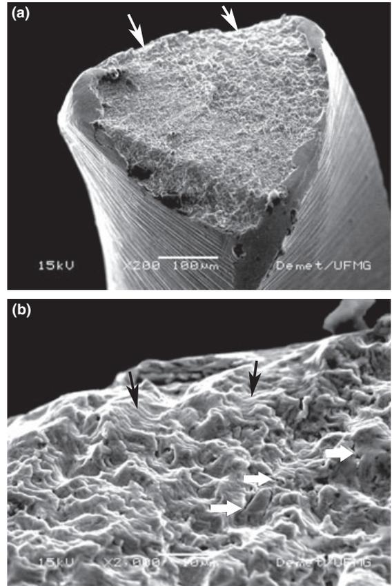
**Figure 4** Fracture surface of a fatigue tested F1 instrument of group C. (a) Smooth regions at the edges of the cross-section (arrowed) and fibrous region at the centre; (b) Detail of the smooth region, showing fatigue striations (dark arrows) and secondary cracks (white arrows).
