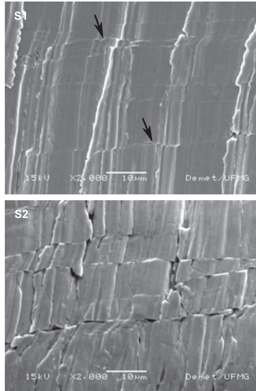
**Figure 2** Typical longitudinal cracks in S1 (arrowed) and S2 instruments used for cleaning and shaping five molars (group A).
