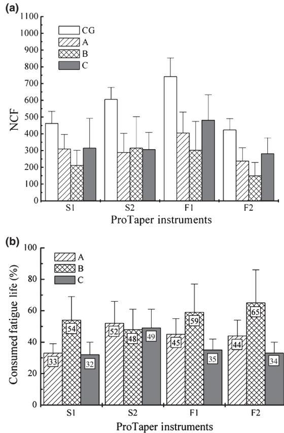
**Figure 3** Mean values of (a) NCF in fatigue tested new ( $n = 12$  for each instrument type) and used instruments ( $n = 10$  for each instrument type) and (b) consumed fatigue life in fatigue tested used instruments; standard deviations shown as error bars.
