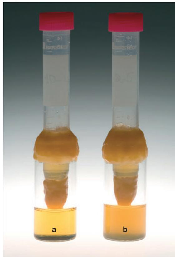
**Figure 1** Two-chamber bacterial leakage test model. a: clear medium in bottom chamber indicating no leakage; b: leaking specimen with bacterial growth in lower chamber.
