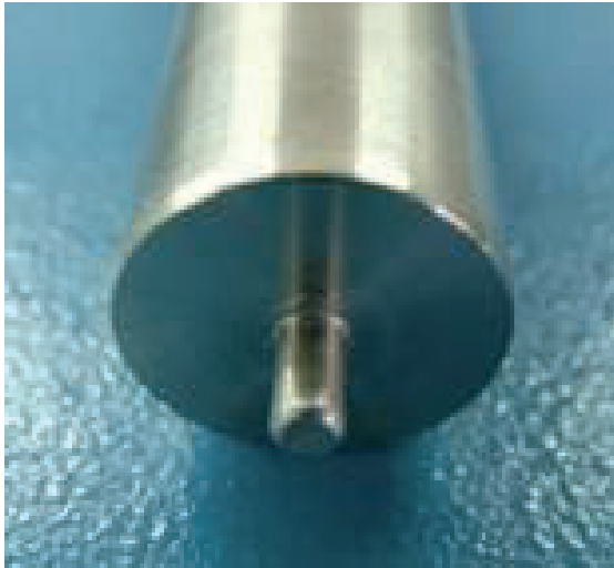
Figure 2 Crosshead tip was used to apply vertical force to the root.
