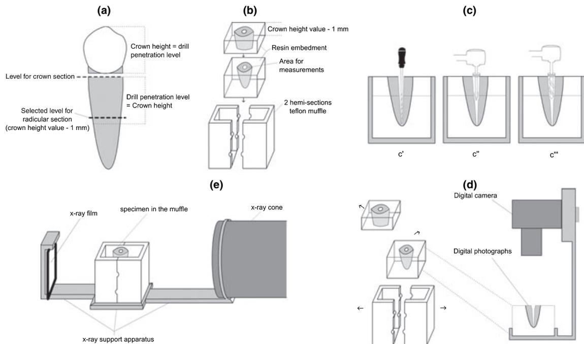
**Figure 1** Schematic illustration of the experimental design used. (a) Tooth preparation and decoronation; (b) root embedment and cross-section; (c) sequence of root canal preparation for post; (c') hand instrumentation; (c'') Gates Glidden drills; (c''') Largo Peeso reamers; (d) muffle disassembling and support apparatus for digital photographs; (e) support apparatus for standardized radiographs.
