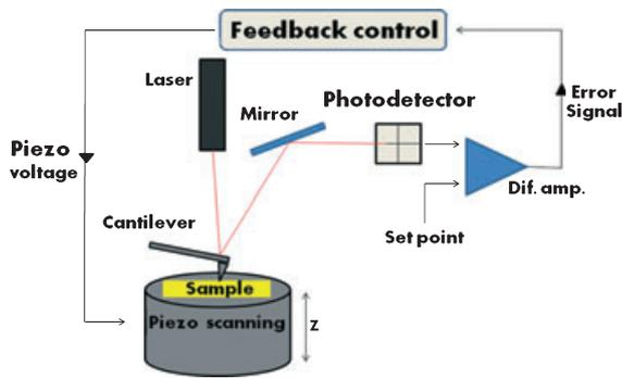
**Figure 1** Schematic representation of the operating principle of an atomic force microscope.
