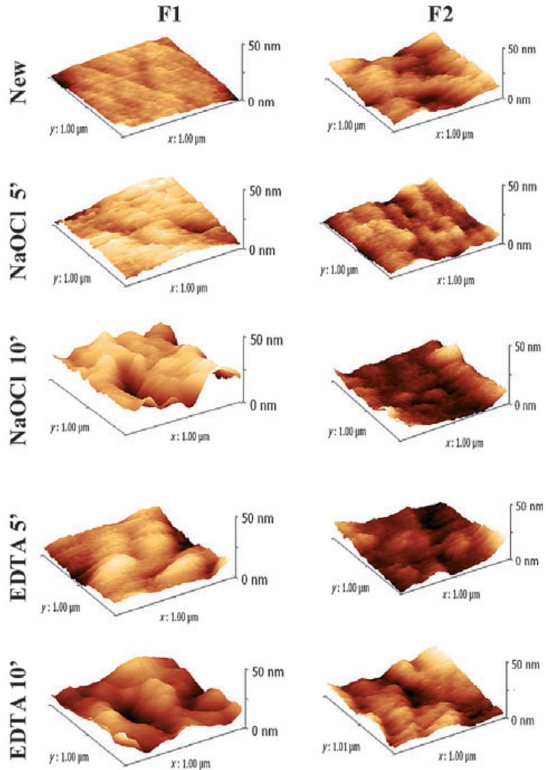
**Figure 3** Three-dimensional atomic force microscopy images of new and immersed ProTaper F1 and F2 instruments.
