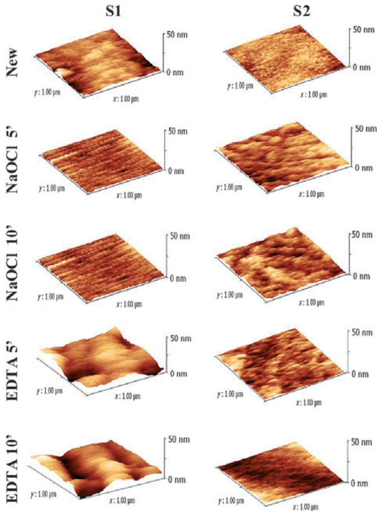
**Figure 2** Three-dimensional atomic force microscopy images of new and immersed ProTaper S1 and S2 instruments.
