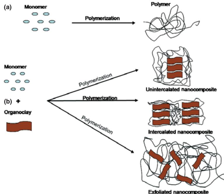
**Figure 2** Incorporation and Levels of dispersion of Organoclay in a polymer matrix. (a) Polymerization of monomer to polymer. (b) Incorporation of Organoclay into monomer and the following polymerization resulting in no dispersion (unintercalated), some dispersion (Intercalation) or high dispersion (exfoliation).
