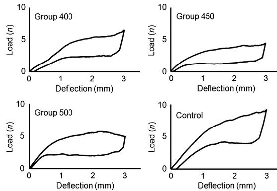
**Figure 1** Typical load–deflection curves for each group.
