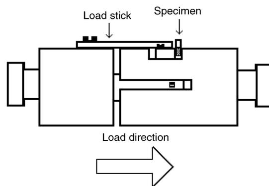
**Fig. 2.** Microshear test apparatus.
