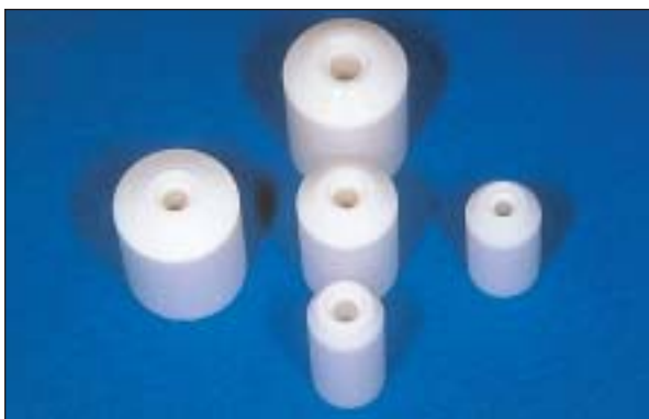
Fig 2 Experimental zirconia abutment ingots with different diameters available for the study.
