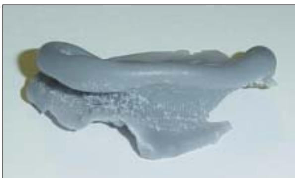
Fig 4 Wax model grown on Thermojet printer.
