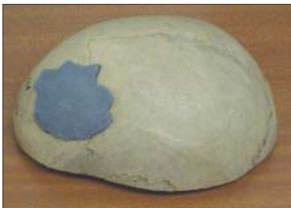
Fig 8 RP-generated skull implant prepared on dry skull specimen.
