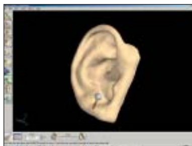
Fig 2 In FreeForm, different tools are chosen to modify image; holes are completed and margin matches deficient side.
