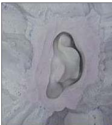
Fig 4b (below) Cavity block formed by vacuum casting.
