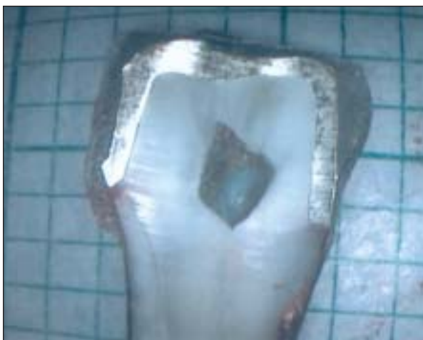
Fig 6 Representative specimen of a tooth section that received MC coping cemented with resin-modified glass-ionomer, after immersion in basic fuchsin solution; original magnification \times 30 .
