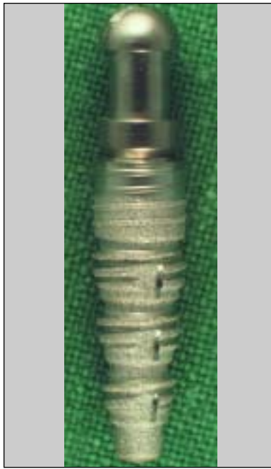
Fig 10a Frialit-2 implant is a stepped, threaded titanium cylinder.
