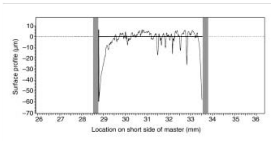
**Fig 3** Profilometric analysis of short side of master 1. Surface shows a few grooves 10 to 20  $\mu\text{m}$  deep, but in general no major alteration in shape.
