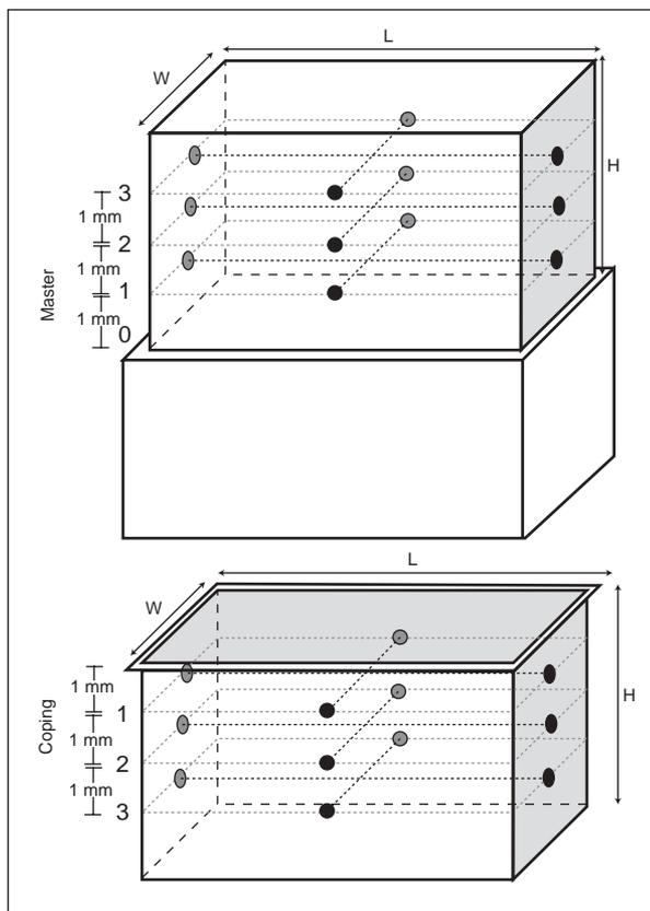
**Fig 2** Measurement points on master model. Height of the master is measured, and other measurements are taken at the midpoints of the width and length dimensions at three levels along the height of the master: 1, 2, and 3 mm.
