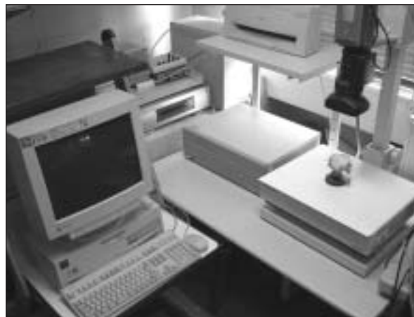
Fig 2 CCD camera, digital image analyzer, and PC used for measurement.
