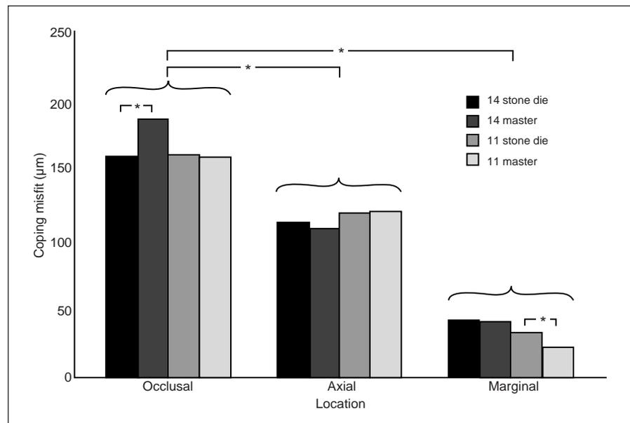
**Fig 4** Mean value of the misfit between Denzir copings and stone die–master model for maxillary right central incisor and first premolar at occlusal, axial, and marginal locations. \* = statistically significant difference with 95% probability.
